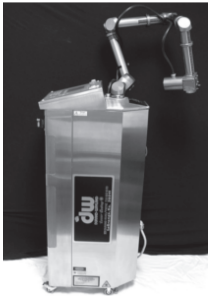
Fig. 1. Laser labeling machine used to etch fruit at the Citrus Research Center's packinghouse in Lake Alfred, Fla. The machine used a maximum energy level of 0.678 W per character at 35 \mu s with a duty cycle range of 25%.
